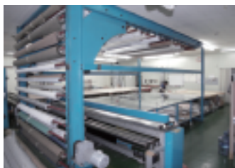
Conveyor- Arch Type
