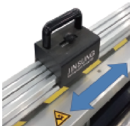
Manual Type Knife & Hand Lever
