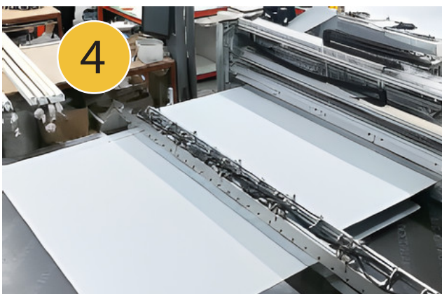
Automatically pull out the fabric
